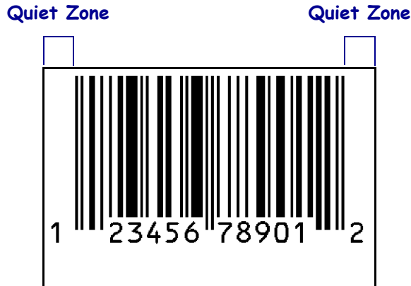
Figure 7 • Quiet Zone in a Bar Code
